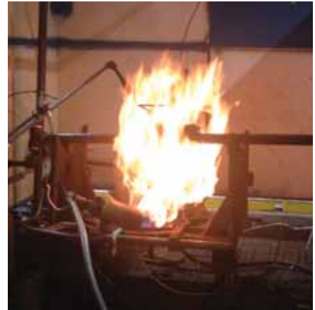
Fire test per API Spec 607 4th Edition.
